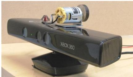
Figure 8: Our simplified setup with a motor hot-melt glued to the Kinect which is mounted on a table with Velcro. A small wooden disc acts as the offset weight.
