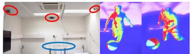
Figure 9: Left: a photo of our setup shows 3 of the ceiling-mounted Kinect cameras (red circles); the extrinsic parameter calibration pattern can also be seen (blue circle). Right: renderings of reconstructed background mesh (lilac) and live foreground mesh of occupant (multi-color).
