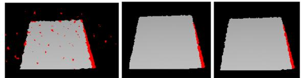
Figure 7: A single, angled plane segmented from background by depth-thresholding. Left: Noisy depth-map with two overlapping patterns. Centre: Ground-truth from single Kinect. Right: Camera shake almost identical to ground-truth.
