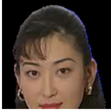
(d) 2x enlarged portion of the reconstructed visual object at 1.0042bpp using SA-DCT coding (PSNR-Y=37.09dB; PSNR-U=42.14dB; PSNR-V=42.36dB).
