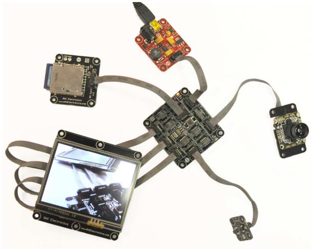
**Figure 4.** An example digital camera built with Gadgeteer.
