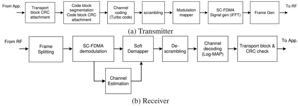
Figure 2: Illustration of LTE PUSCH transceiver.
