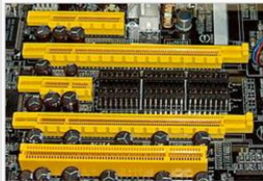
PCI Express slots (from top to bottom: \times 4 , \times 16 , \times 1 and \times 16 ), compared to a traditional 32-bit PCI slot (bottom), as seen on DFI's LanParty nF4 SLI-DR.
