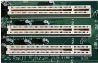
Three 5 V 32-bit PCI expansion slots on a motherboard (PC bracket to left)
