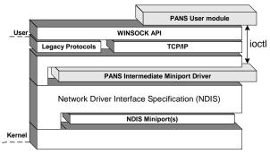
**Figure 2**: The network protocol stack showing the PANS Intermediate driver and its location in the NDIS stack. The PANS user module runs at the application level and communicates with the driver using *ioctl* calls.
