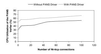
**Figure 7**: The CPU Utilization of the PANS Verifier as a function of the number of ntttcp connections. On average, the CPU utilization increases by 40% in the presence of the PANS Intermediate driver.
