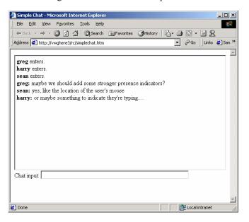
The SimpleChat implementation consists of a <span> that contains all of the text history, embedded in a <div> that provides the scrollbars, plus one <div> for each userentered comment. The history <span> is defined as:
