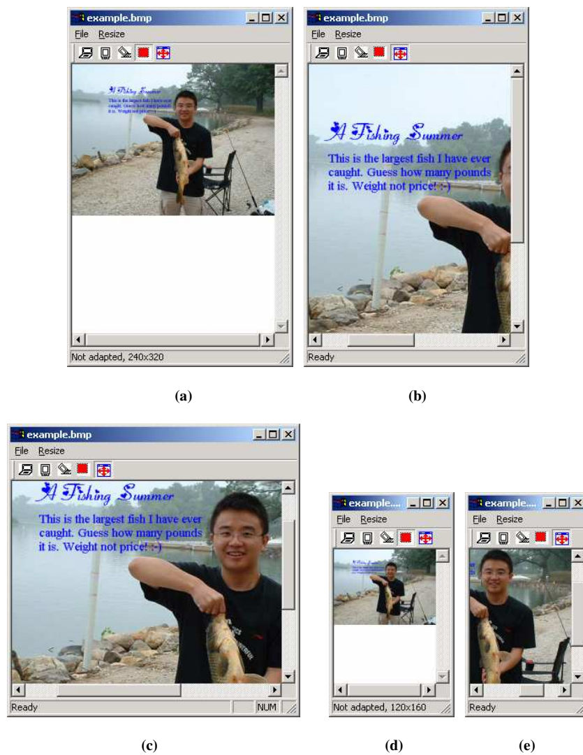
Fig. 11. An example comparing the proposed attention model with the conventional approaches to adapt image. (a) direct down-sampling for Pocket PC, (b) attention-based method for Pocket PC, (c) a better adapted result by rotation for Pocket PC, (d) direct down-sampling for Smartphone, and (e) attention-based method for Smartphone
