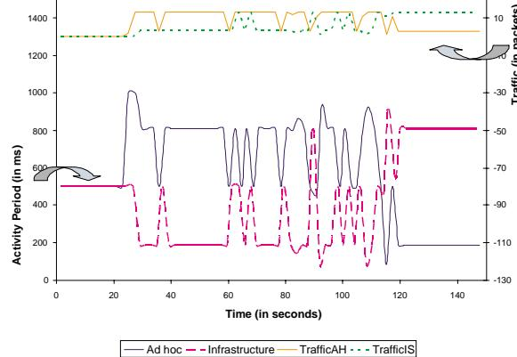
Fig. 9. Variation of the activity period for two networks with time. The activity period of a network is directly proportional to the relative traffic on it.
