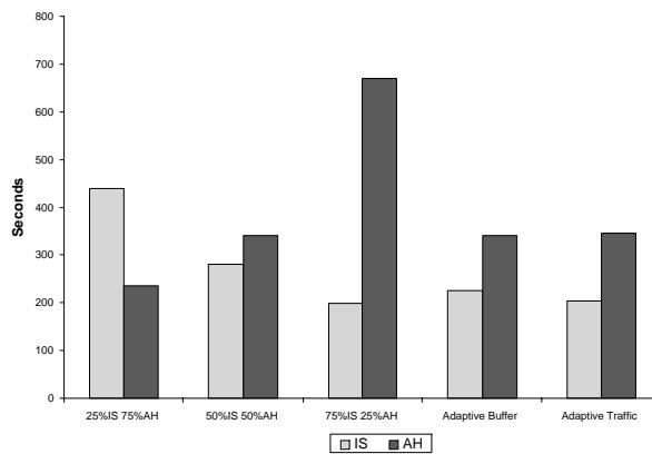
Fig. 8. Amount of time taken to complete the FTP transfer of a file on an ad hoc and infrastructure network for different switching strategies
