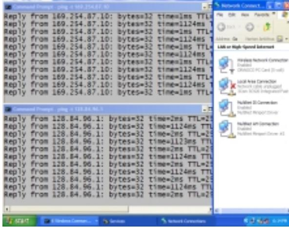
Fig. 5. A screen snapshot of a MultiNet node connected to two networks using legacy 802.11 cards
