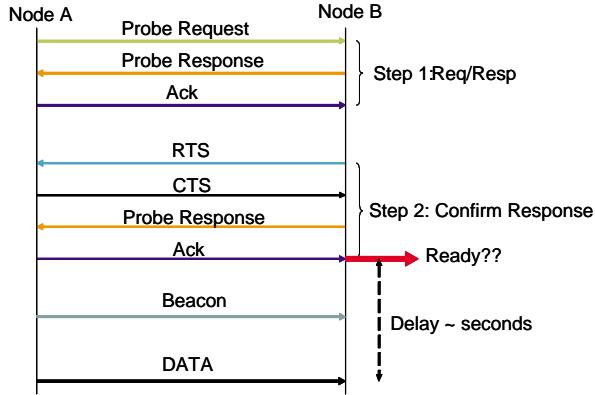
Fig. 6. Message exchange, as seen by AiroPeek, when switching to an ad hoc network on the Cisco 340 Series wireless adapter
