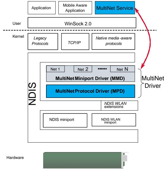
Fig. 4. The modified Windows network stack
