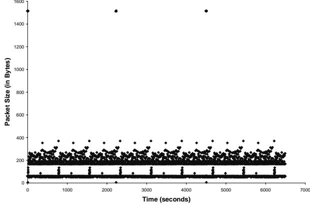
Fig. 12. Packet trace for the presentation and chat workloads over the ad hoc network
