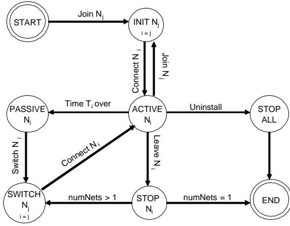
Fig. 3. The states of a MultiNet node
