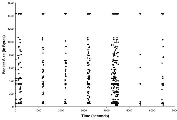
Fig. 11. Packet trace for the web browsing application over the infrastructure network
