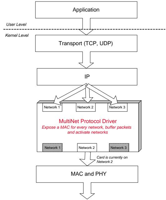
Fig. 1. Modified network stack
