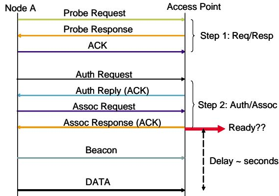
Fig. 7. Message exchange, as seen by AiroPeek, when switching to an infrastructure network on the Cisco 340 Series wireless adapter
