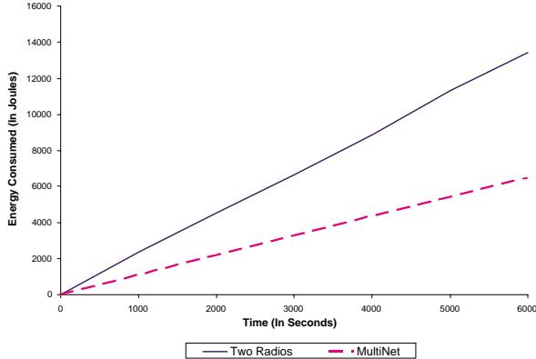
Fig. 13. Comparison of total energy usage when using MultiNet versus two radios
