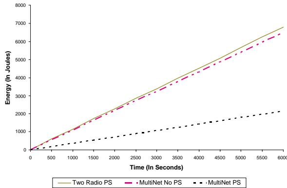
Fig. 14. Energy usage when using MultiNet and two radios with IEEE 802.11 Power Saving
