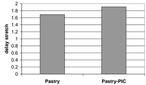
Fig. 12. Delay stretch in a 20,000-node Pastry overlay in GATech with and without PIC.
