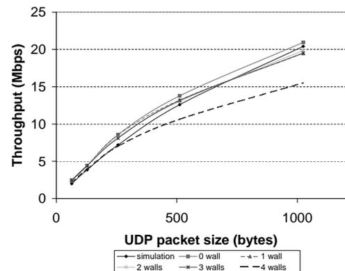
**Figure 6: Estimated throughput matches with measured throughput when the RF condition of the links is good, and deviates when the RF condition of the links is poor (1-hop connection).**
