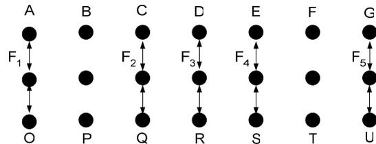
Figure 3: The flow  $F_3$  gets a much higher share of the bandwidth than the flows  $F_2$  and  $F_4$ , even though all the flows have the same application-level sending rate. A simple heuristic may conclude that nodes D and R are misbehaving, whereas simulation can correctly determine the observed throughput is expected.
