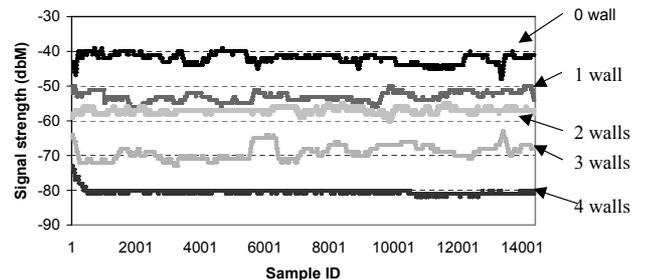
**Figure 7: In good environmental conditions, received signal strength remains stable over time.**
