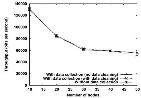
Figure 13: Effect of overhead on throughput
