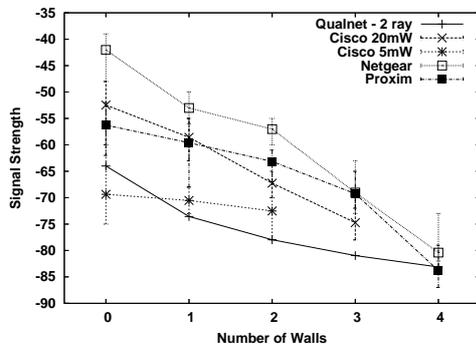
**Figure 4: Comparing the simulator's two-ray RF wave propagation model for received signal strength with measurements taken from IEEE 802.11a WLAN cards from different hardware vendors.**
