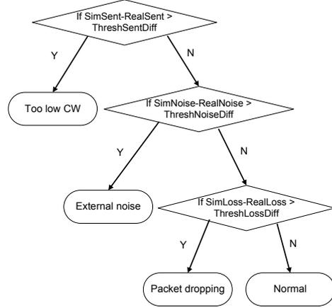
Figure 10: An algorithm to determine the type of faults
