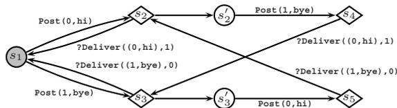
**Fig. 1.** Sample test graph generated by Spec Explorer from the chat model; diamonds represent passive states; ovals represent active states; links to  $s'_2$  and  $s'_3$  represent transitions to active mode; observable actions are prefixed by a question mark.
