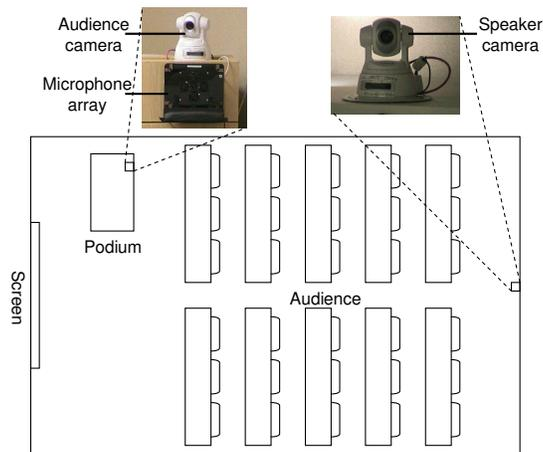
Fig. 4. A typical configuration of the *iCam2* system.
