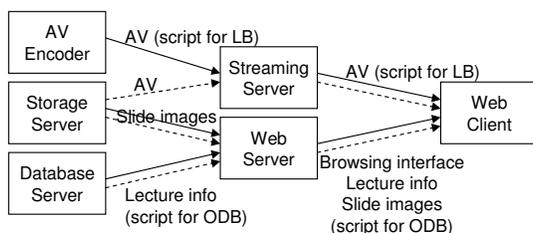
Fig. 2. Live and on-demand broadcasting diagram. The solid arrows are data flow for live broadcasting (LB), and the dash arrows are data flow for on-demand broadcasting(ODB).
