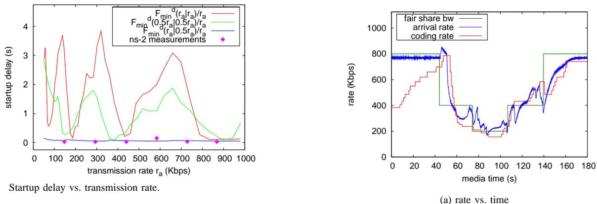
Fig. 20. Startup delay vs. transmission rate.
