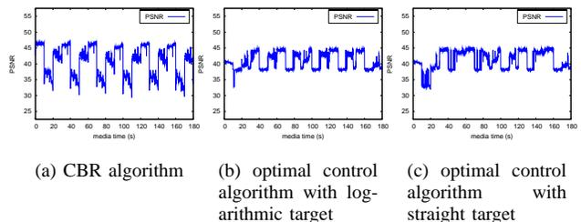
Fig. 34. PSNR with constant bandwidth (400 Kbps) over TFRC.
