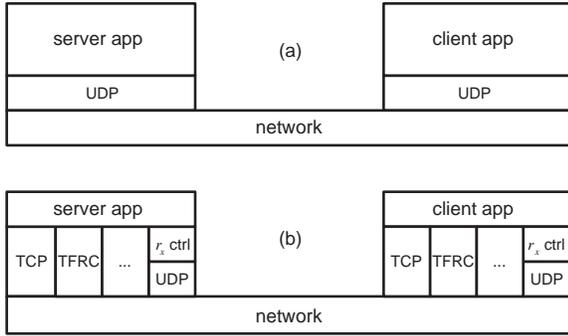
Fig. 1. (a) Traditional streaming media architecture. (b) Proposed streaming media architecture with congestion control factored out.
