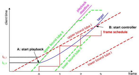
Fig. 16. Leaky buckets (buffer tubes) for various transmission rates.
