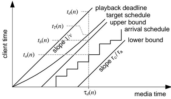
Fig. 5. Arrival schedule and its upper bound in client time. The upper bound is controlled to the target schedule, which is increasingly in advance of the playback deadline to provide greater robustness over time.
