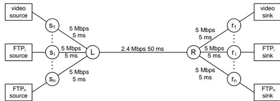
Fig. 19. ns-2 Simulation network setup.
