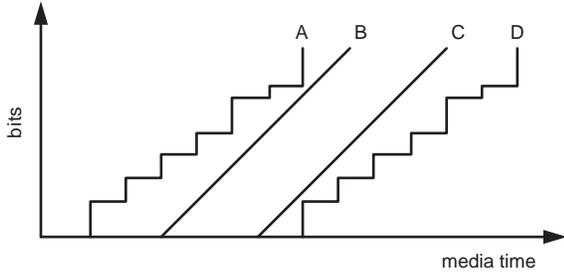
Fig. 3. Schedules at which bits in the coded bit stream pass the points A, B, C, and D in the communication pipeline.
