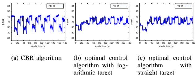
Fig. 33. PSNR with constant bandwidth (400 Kbps) over TCP.
