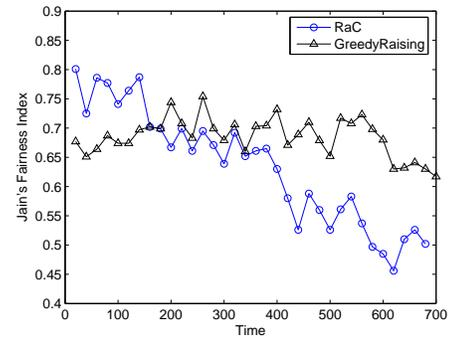
Fig. 11. Fairness Index of 160 clients in a 25 AP WLAN when aggregated over 20 second intervals over 700 seconds.
