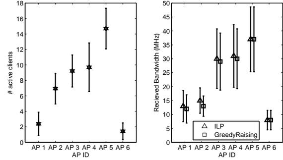
Fig. 8. Average number of clients associated to each AP and the corresponding bandwidth allocated by our scheme.
