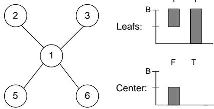
Fig. 2. Network in which a throughput-optimal solution is unfair. T and F denote the allocations in a throughput-optimal and fair solution, respectively.
