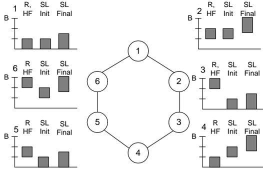
Fig. 4. Ring network with bandwidth options  $B/2$  and  $B/3$  and uniform load. The smallest-last (SL) packing heuristic performs better ( $L_{Sys} = 3B$ ) than the heavy-first (HF) and random (R) heuristics ( $L_{Sys} = 2B$ ). In the example, the ordering of HF and R is  $\mathcal{O} = (1, 4, 2, 3, 5, 6)$ .
