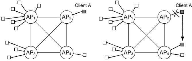
Fig. 1. A network with four mutually interfering APs. With fixed channel bandwidths, both throughput and fairness is suboptimal.
