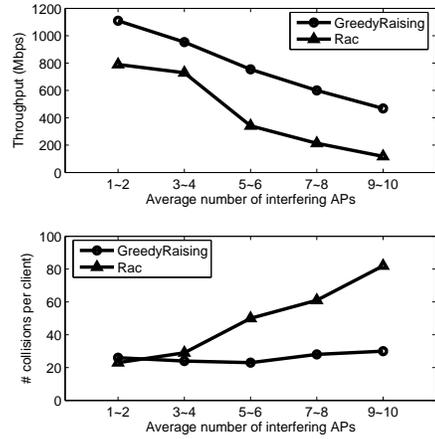
Fig. 10. System throughput and per-client collisions in a WLAN of 50 APs
