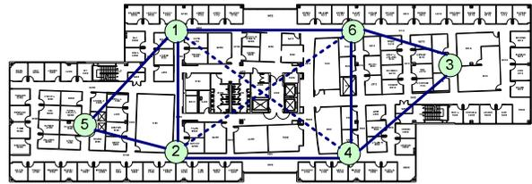
Fig. 5. Floor plan and AP locations on the floor of an office building. The solid lines represent two interfering APs, and dashed lines indicate that the APs interfere at one of the clients.
