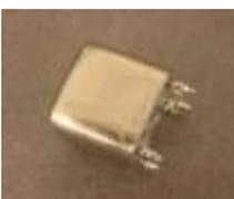
The gyro used is the Gyration MG1101 MicroGyro. It contains two axes of measurement and operates over a 2-wire serial bus. In this project, we placed the gyro inside and at the base of the walking stick prototype, shown at right. The gyro measures the angular velocity of the walking stick.
