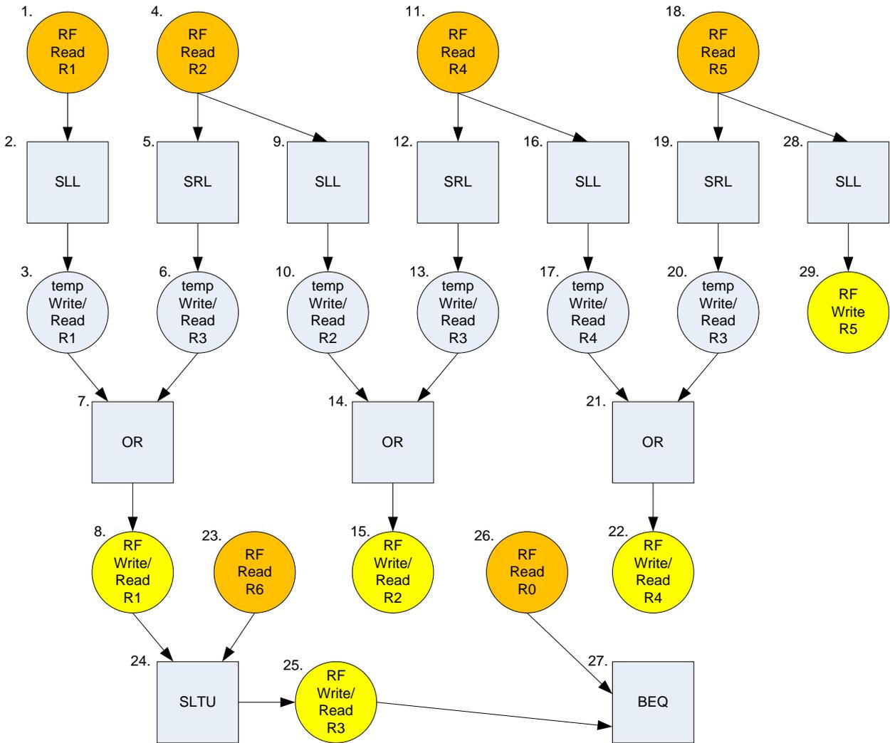
Figure 3: Dependency graph for the basic block in Figure 1.
