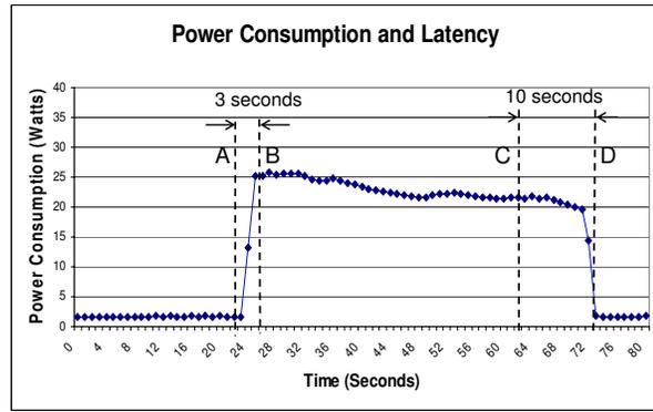
**Figure 6: Power consumption of the entire system during operation. A laptop wakeup event occurs at point A and the machine is fully resumed by point B. At point C a suspend to RAM request is made, which completes at point D.**
