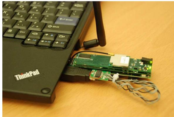
**Figure 5: Photo of Somniloquy prototype. The gumstix can be seen connected to one USB port while the custom PCB with the FTDI chip is connected to the other USB port on the laptop.**
