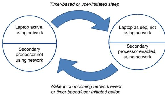
**Figure 1: High-level operation of Somniloquy.** The secondary processor actively uses the network when the laptop is asleep. At any time, only one of the laptop or the secondary processor is actively using the network.
