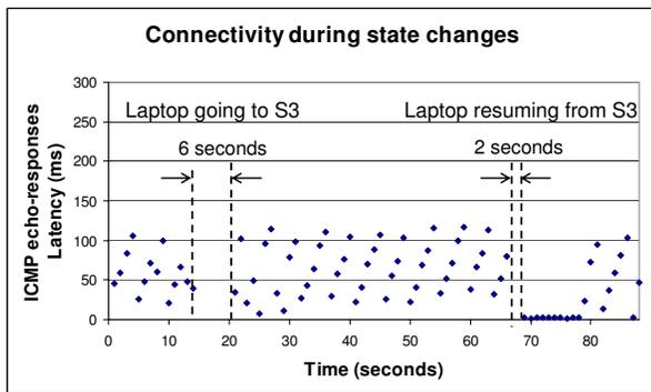
**Figure 7: ICMP echo-response (ping) trace for prototype going into S3 and subsequently resuming from S3.**
