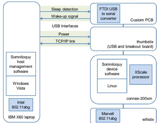
**Figure 4: Block diagram of the Somniloquy prototype system. The figure shows various components of the gumstix and the USB interfaces to the host laptop.**
