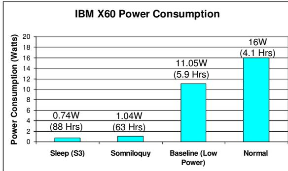
Figure 8: Power consumption and the resulting estimated battery lifetime of an Lenovo X60 using Somniloquy. The lifetime is calculated using the standard 65 Watt hour battery of the laptop.
