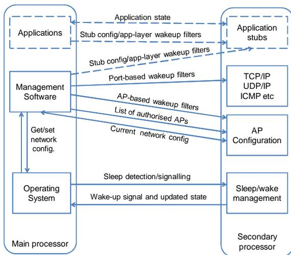
**Figure 3: Somniloquy software components on the laptop and the secondary processor, and their interactions. The dotted lines represent components that have not been completely implemented, but are nice to have.**
