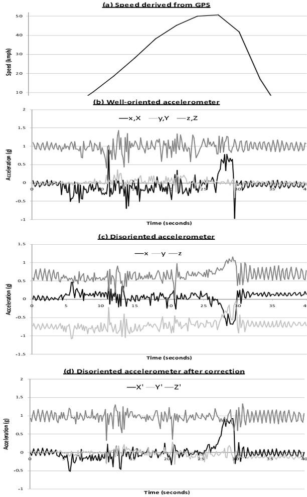
Figure 4: Estimating the orientation of a disoriented accelerometer based on sharp deceleration starting at around 27 seconds:  $\phi_{pre} = -88^\circ$ ,  $\theta_{tilt} = 49^\circ$ ,  $\psi_{post} = -135^\circ$
