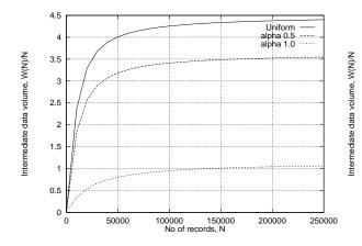
Figure 3: Intermediate data volume as a function of input size when using repeated scanning. 10,000 groups, 10% in memory.
