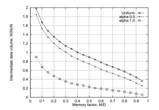
Figure 11: Intermediate data volume as a function of memory size when using sorting with run formation by load and sort. 10,000 groups, 1,000,000 input records, fan in 10.
