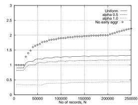
Figure 10: Intermediate data volume as a function of input size for grouping by sorting with run formation by replacement selection and using an optimal merge pattern. 10,000 groups, 10% in memory, fan in 10.
