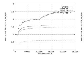
Figure 9: Intermediate data volume as a function of input size for grouping by sorting with run formation by load and sort and using an optimal merge pattern. 10,000 groups, 10% in memory, fan in 10.
