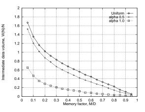
Figure 12: Intermediate data volume as a function of memory size when using sorting with run formation by replacement selection. 10,000 groups, 1,000,000 input records, fan in 10.
