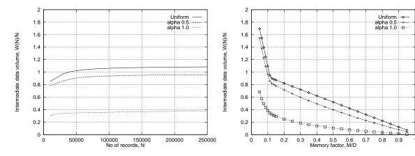
Figure 13: Intermediate data volume as a function of input size when using simple partitioning. 10,000 groups, 10% in memory, 10 partitions, buffer size 25 records.
