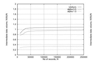
Figure 15: Intermediate data volume as a function of input size when partitioning partially aggregated records. 10,000 groups, 10% in memory, page size 25 records, min 5 pages/partition.
