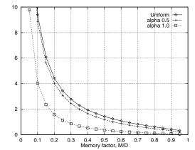
Figure 6: Intermediate data volume as a function of memory size when using repeated union with aggregation. 10,000 groups, 1,000,000 input records.
