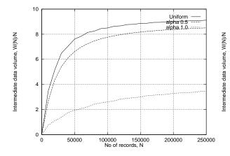
Figure 5: Intermediate data volume as a function of input size when using repeated unioun with aggregation. 10,000 groups, 10% in memory.
