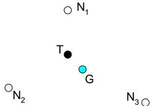
**Figure 4** An illustration of how averaging multiple nearest neighbors ( $N_1, N_2, N_3$ ) can lead to a guess (G) that is closer to the user's true location (T) than any of the neighbors is individually.
