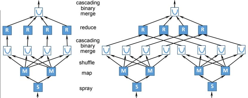
**Figure 3: Two-stage streaming temporal map-reduce (one and two inputs).**
