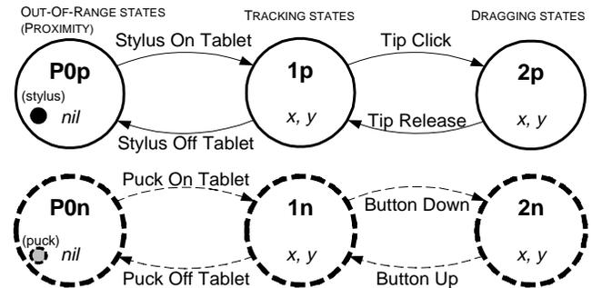
Fig. 11 Simple model for puck and stylus on the tablet. The tokens start in states  $P0_p$  and  $P0_n$ , indicating that neither device is in proximity. We label the tokens here for clarity.
