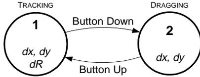
Fig. 7 The IntelliMouse. We omit  $dR$  from state 2 because it is difficult to turn the wheel while dragging the mouse. This precludes some useful transactions, such as scrolling a document while dragging a figure into place.
