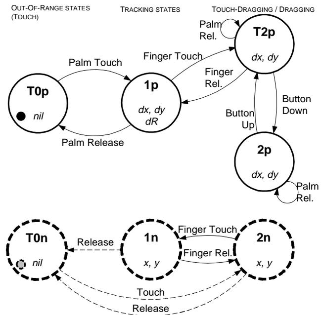
Fig. 15 Adding state  $1_n$  to the device states to support both cursor tracking and dragging with the touchpad.
