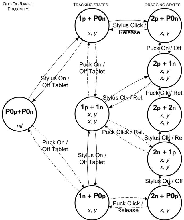
Fig. 10 Full state model for Wacom puck and stylus. The dashed arcs show events for the puck, solid arcs events for the stylus. It is hard to see how this model corresponds to the individual 3-state models for the puck and stylus.
