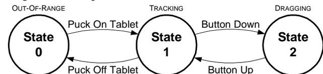
Fig. 3 State transitions for the puck on the Wacom tablet.
