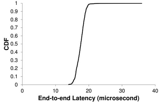
Figure 8: End-to-end delay of  $\mu$ ACK feedback.
