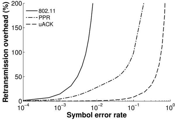
**Figure 5: Retransmission overhead versus the symbol loss rate on the wireless link. The packet size is 1500B and the data rate is 54Mbps.**
