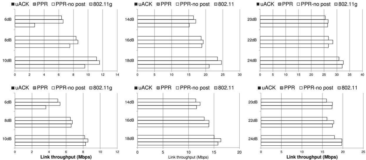
**Figure 12: Link throughput of three schemes under different SNR. Top row: packet size is 1500B. Bottom row: packet size is 500B. Left: Low SNR regime. Middle: Middle SNR regime. Right: High SNR regime. X-axis Y-axis shows the SNR (dB).**
