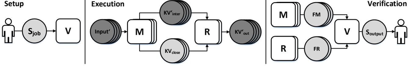
**Fig. 4:** Schematic overview of our job execution protocol. The verifier (**V**), mappers (**M**), and reducers (**R**) are depicted as squares. A light-gray circle displays a message/key-value pair that is sent *once* by an entity; a dark-gray circle one that is sent multiple times. The user is depicted at both far ends.
