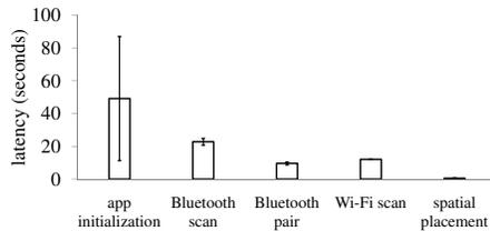
Fig. 15: This graph shows the latency of various tasks in Virtual Compass, along with error bars indicating variance across several runs. A total of 10 stationary devices were placed in a  $100m^2$  area. “app initialization” is dominated by communication with the Facebook Web site.
