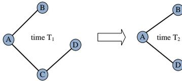
Fig. 3: An example illustrating the calculation of the change metric for adapting the Bluetooth scan interval. In this example, the change metric between  $T_1$  and  $T_2$  is 1.9, which is high enough to trigger a reduction in the scan interval.
