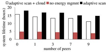
Fig. 13: This graph shows the lifetime of Virtual Compass on a fully-charged stationary mobile phone, with different energy conservation techniques and different numbers of nearby peer devices in a  $100m^2$  area. In this experiment, the devices did not move.
