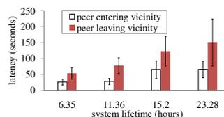
Fig. 17: This graph shows the trade-off between the latency of detecting a peer moving into or moving out of the vicinity, against the lifetime of Virtual Compass . We varied the Wi-Fi scan interval between 30 seconds and 4 minutes.
