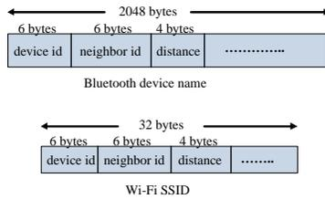
Fig. 7: Packet format for beacons in Virtual Compass
