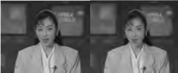
Figure 2: Akiyo frame 11 encoded at 20 kbps using 3-D ESCOT (left) and 3-D SPIHT (right).
