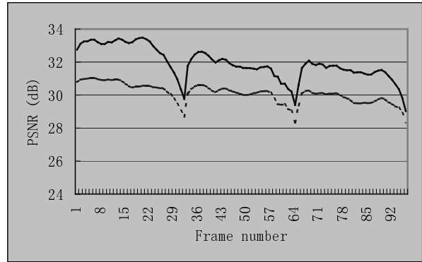
Figure 3: PSNR vs. frame number (1-96) for "Mother & Daughter" at 20kbps by 3-D ESCOT (solid line) and 3-D SPIHT (dash line).
