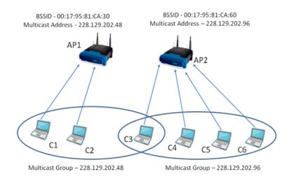
Figure 3: Improving User Association in WLAN using Neighborcast
