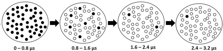
Figure 7: Chained Contention Resolution Example in WiFi-Nano
