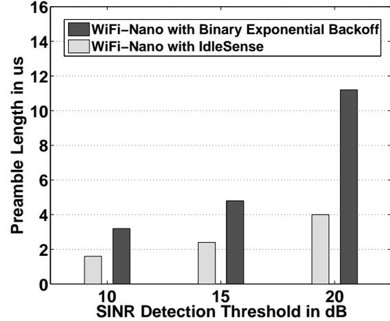
Figure 13: Preamble length for different detection thresholds
