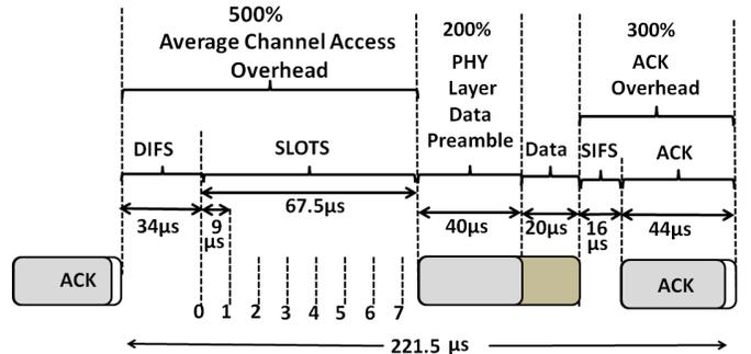
Figure 1: Overheads in 802.11 at 600 Mbps
