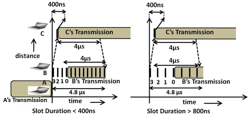
Figure 5: Design of slot width in WiFi-Nano
