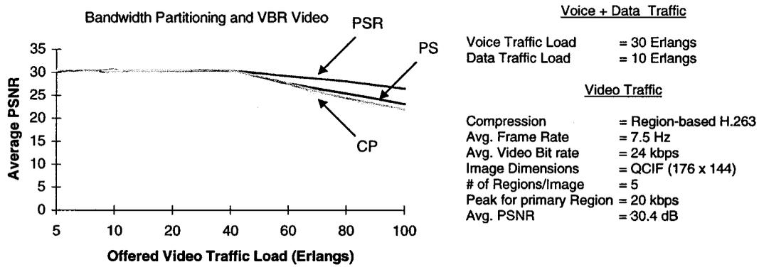
Figure 4. Comparison of bandwidth partitioning schemes
