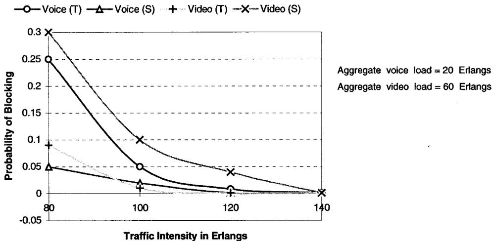
Figure 7. Performance of load-proportional approach with VBR video
