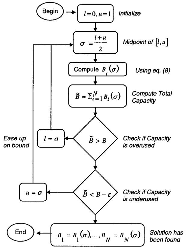
Figure 6. Algorithm *Smart Allocate*
