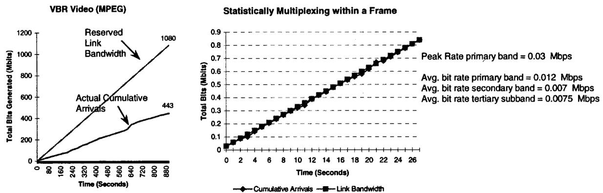
Figure 2. Bandwidth utilization for VBR video with and without intra-frame statistical multiplexing
