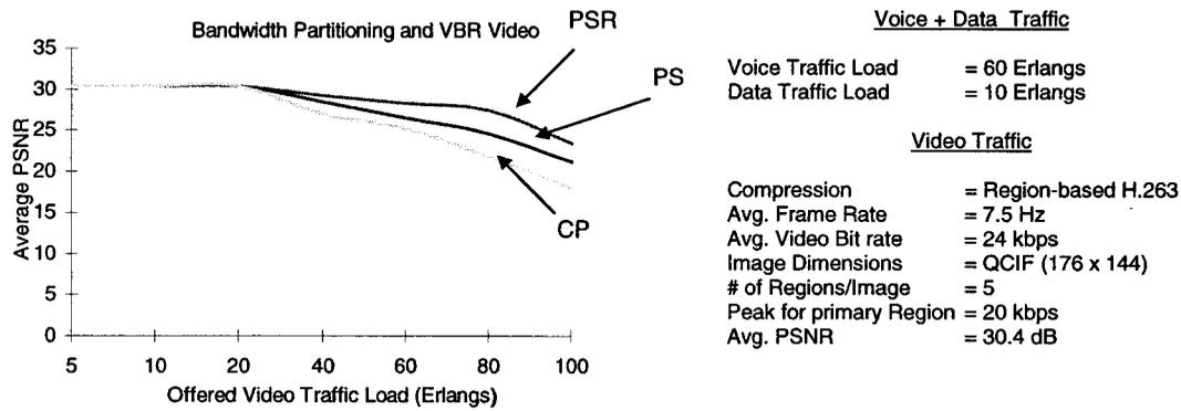
Figure 5. PSR performance with increased voice traffic
