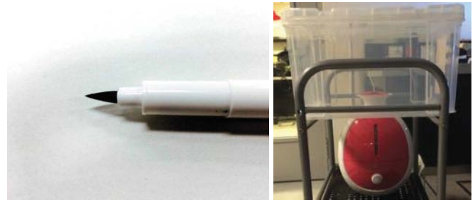
(a) Silver nano particle ink filled AgIC brush/marker
