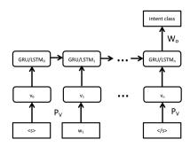
Fig. 3. Proposed LSTM/GRU classifier model.
