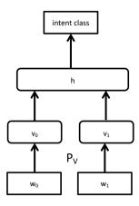
**Fig. 1**. The standard Neural Network Language Model.  $P_w$ , the projection layer, is shared by  $\mathbf{w_1}$  and  $\mathbf{w_2}$ . Word embeddings from those words,  $v_1$ ,  $v_2$ , are stacked into a single vector, which serves as input to a multilayer perceptron. In this architecture, the NNLM is predicting the next word, but can also predict other labels, such as addressee labels.
