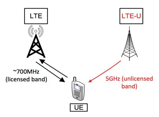
LTE-U: Control channel in licensed band and supplemental downlink data channel in unlicensed band (5GHz)
