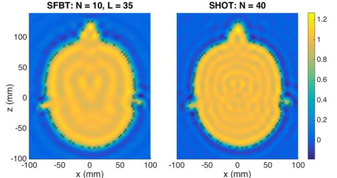
**Fig. 2.** Head shape reconstruction on a horizontal plane passing through the interaural axis, for a) SFBT, and b) SHOT. The dots represent the actual intersection points on the boundary of the mesh returned by the raytracer.
