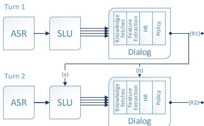
Figure 1: Schematic diagram of the experimental spoken dialog system where (a) is a domain only contextual signal, (b) is the domain, intent and entities contextual signals, (R1) is selected result of turn 1, (R2) is selected result of turn 2.
