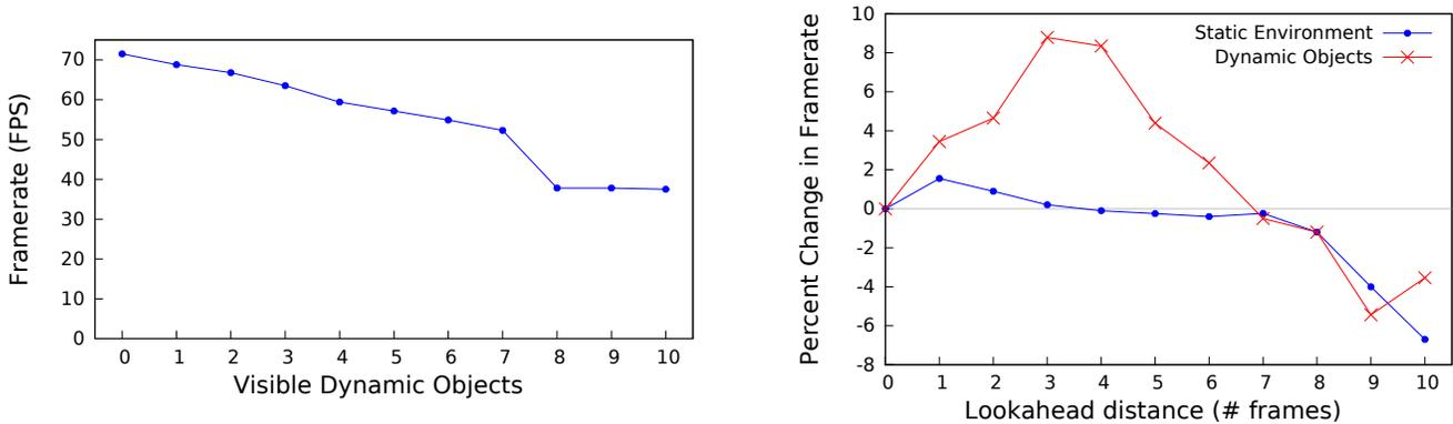
**Figure 13:** FLASHBACK scales well to a moderate number of visible dynamic objects, maintaining a high framerate until insufficient memory causes page thrashing.
