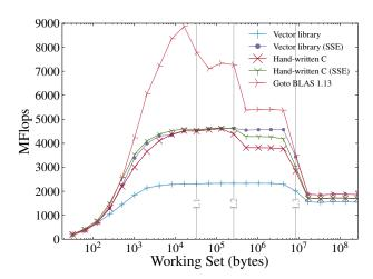
Figure 5: Single-threaded performance of double-precision dot product implementations. C implementations were compiled using GCC 4.8.1 and compiler options -03 -msse4.2 -ffast-math -ftree-vectorize -funroll-loops. Sizes of the L1, L2, and L3 caches are marked.
