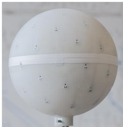
Fig. 1. 64-channel spherical microphone array.
