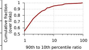
Figure 1: Ratio of 90<sup>th</sup> percentile to 10<sup>th</sup> percentile link utilization shown as a cumulative distribution function.
