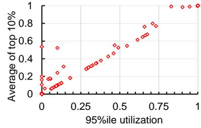
**Figure 5:** Scatter plot of 95<sup>th</sup> percentile and average of top 10% utilization values. Each point corresponds to a link.
