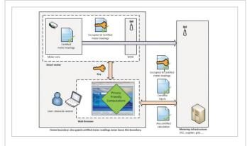
Many smart metering systems threaten users' privacy by disclosing data about consumption to utility companies, e.g. power suppliers. We have designed a system that allows for precise billing of consumption while not revealing any consumption information to utility companies.
