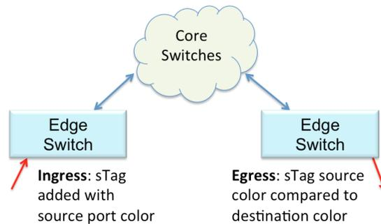
Figure 4: A Sample sTag Deployment.
