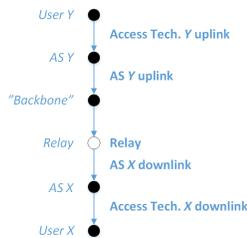
**Figure 3: Topology for bandwidth, jitter, and loss metrics. Logical entities are shown in italics on the left with the resulting modeling components in bold-face type on the right.**
