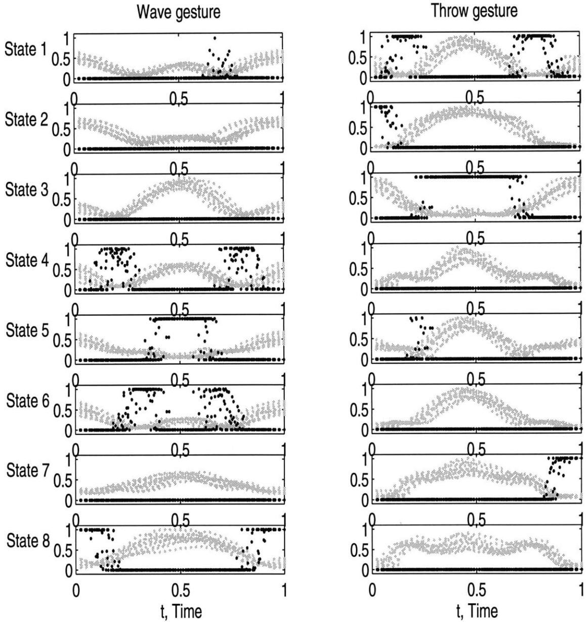
**Figure 5-3:** Plots of  $\gamma_{t_i}(j)$  (black) and  $d_m$  (gray) for two gestures trained concurrently. The plots of  $\gamma_{t_i}(j)$  indicate that the states were divided evenly over the gestures (four states for each gesture), though some states are briefly shared (states 1 and 5). ( $d_m$  was scaled to fit.)
