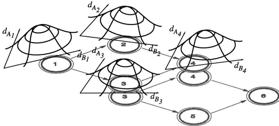
**Figure 5-1:** Two different gestures are associated with unique Markov models (gray), but share observation distributions at states 3 and 4.
