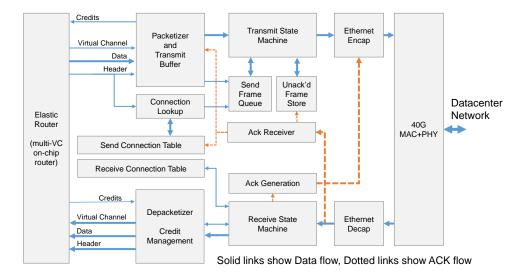
Fig. 9. Block diagram of the LTL Protocol Engine.
