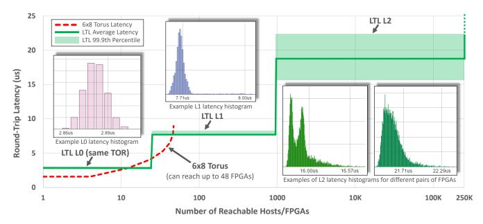
Fig. 10. Round-trip latency of accesses to remote machines with LTL compared to the 6x8 torus from [4]. Shaded areas represent range of latencies up to the 99.9th percentile. LTL enables round-trip access to 100,000+ machines in under 23.5  $\mu$ s.
