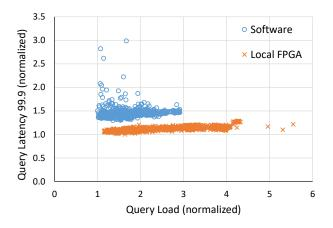
Fig. 8. Query 99.9% Latency vs. Offered Load.
