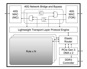
Fig. 4. The Shell Architecture in a Single FPGA.
