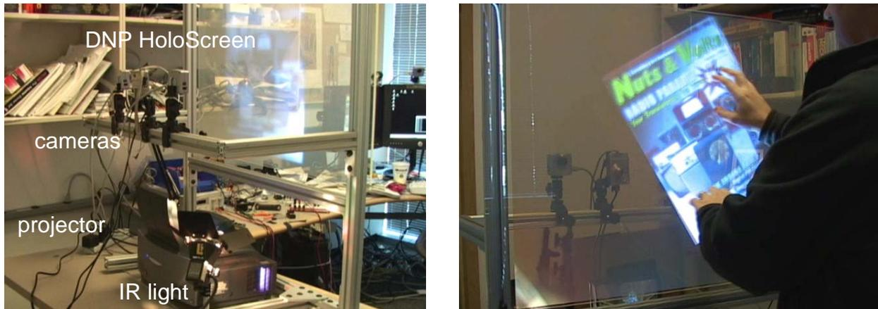
**Figure 4** TouchLight prototype. Left: Placement of video cameras directly behind HoloScreen, short-throw projector, and infrared light. Right: High resolution still capture of magazine cover placed on the display surface is directly manipulated by hand motion.
