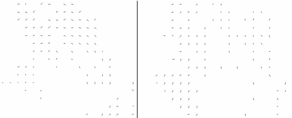
**Figure 2** Flow fields represent more than translation. Left: Flow field generated by clockwise rotation of the hand. Note how the flow field vectors lie along circles about the point of rotation. Right: Flow field generated by hand raising over keyboard. Here the flow vectors indicate an expansion about a point.
