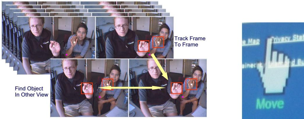
**Figure 3** GWindows. Left: Illustration of stereo image processing to find moving, hand-sized objects in the scene. Only the nearest such object is labeled as the hand. Right: On-screen representation of hand position.
