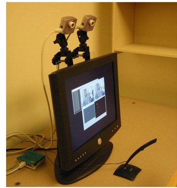
Figure 4: Experimental Setup. Study participants were seated in front of a GWINDOWS-enabled display and an open microphone for speech recognition.
