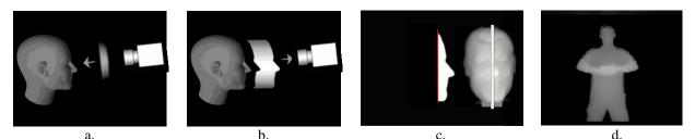
Figure 1. 3DV ZSense uses pulsed infrared light (a) and solid state shutter to compute depth image. Reflected light from closer surfaces arrives sooner (b). Fast shutter truncates light (c) while imaging sensor integrates more light from closer surfaces. A second captured image is used to normalize for differences in reflectance. Example depth image (d). Illustrations adapted from [1].
