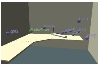
**Figure 3**: A 3-d graphics visualization of the wand world model with several trained targets in an office space. The wand (foreground) is shown as a white cylinder and coordinate axes.
