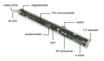
Figure 1: XWand hardware prototype.
