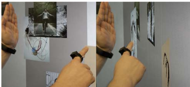
Figure 5. Example of ChopZ. Left: Using right hand to select scope after chop with left hand. Right: Using right hand to move individual elements to change visual stacking order.
