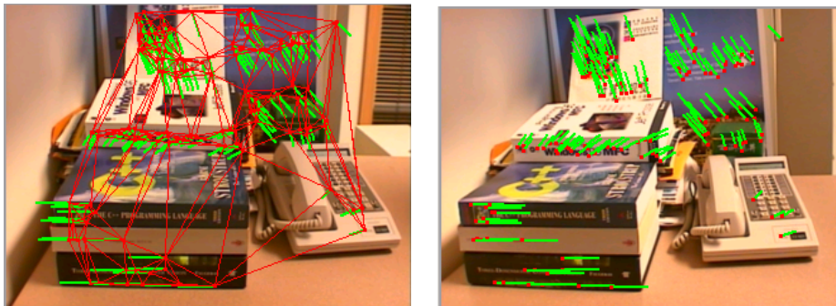
Fig. 4. Scene Books : Initial point matches indicated by the disparity vectors together with the Delaunay triangulation in the first image.
