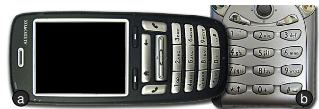
Figure 6. (a) The Audiovox 5600 phone. (b) The Red-E SC1100 phone offers more space between buttons.
